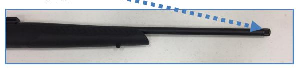
MOUNTING STEP #2: The threaded part of the firearm barrel should now be visible on your firearm. The <a href="thread should be 1/2x28">thread should be 1/2x28</a> in order to be compatible with your Boomhusher 5.56mm Suppressor
