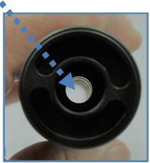
MOUNTING STEP #5: Align the threaded muzzle cap with the threaded portion of the muzzle. Thread the suppressor onto the barrel by rotating in a clockwise fashion until shouldered onto the barrel of the host firearm. Hand-tighten only, do NOT tighten with a wrench of any kind. If threading becomes difficult, then stop and unthread the suppressor off of the barrel to prevent cross-threading. Check that the threads are clean and re-attempt.
